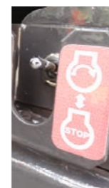
Emergency engine stop switch
