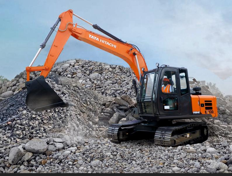
Engine Power: 76 PS @ 2200 rpm
