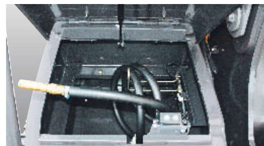
Electric fuel refilling pump
