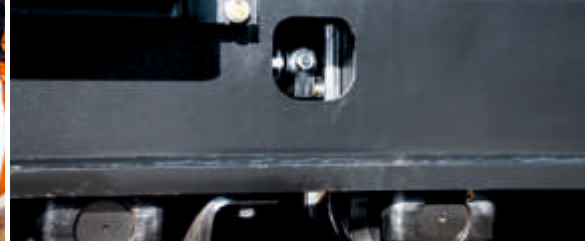
Adjuster greasing hole repositioned to reduce dirt accumulation
