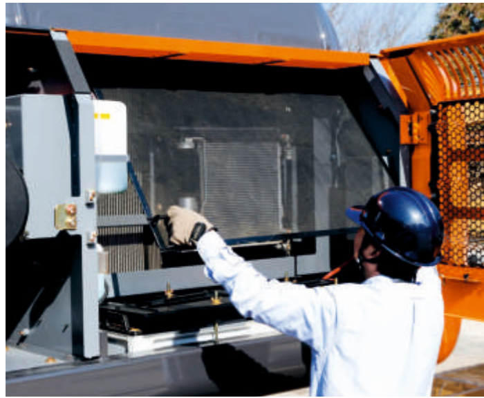
Easily detachable dust-proof indoor net
