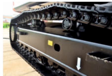
45 Ton class heavy duty track frame
